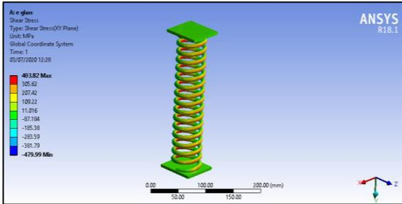
Figure 4: Shear Stress generated using E-glass material
