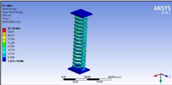
Figure 5: Strain energy using E-glass material
